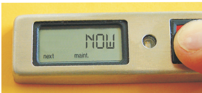
display showing the maintenance is due now
